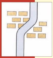
The flue is the passage in the chimney through which the combustion gasses pass to the atmosphere. Ideally it should be the same dimensions from just above the throat to the base of the chimney pot, although in some cases it will change direction for constructional reasons.
