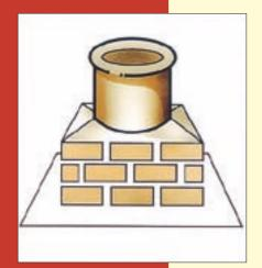
It is absolutely essential to make an external check on the condition of the chimney in the roof space and above roof level. Ensure the mortar joints are intact and that the structure is vertical.
